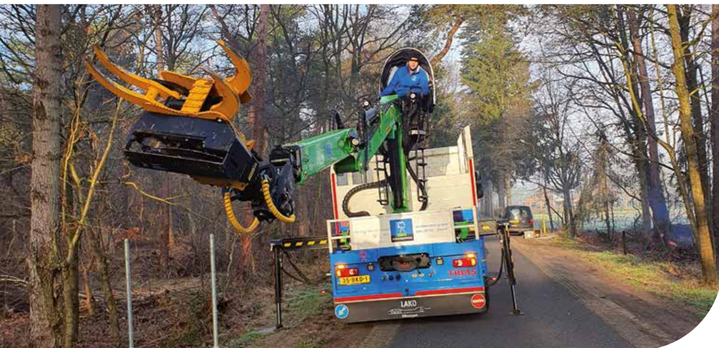
Truck with GMT035TTC grapple saw and GMT C10 quick coupler system
