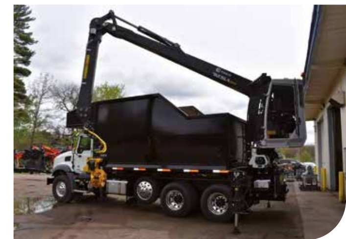
GMT050TTC with a crane point adapter for a forestry crane
