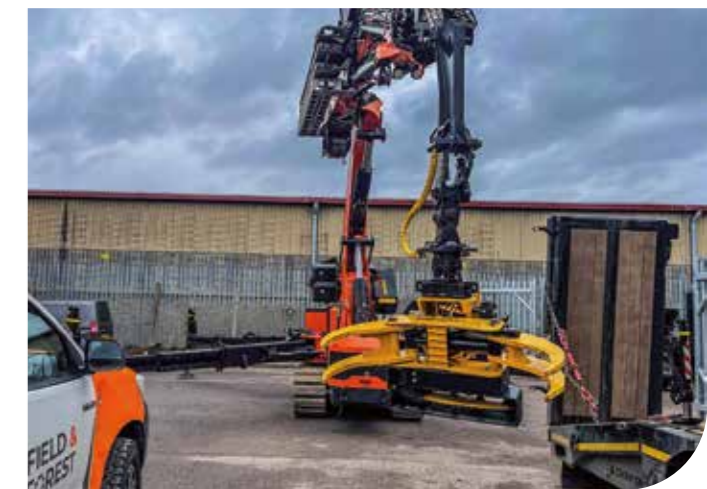
GMT050TTC with an extension arm for a crawler crane
