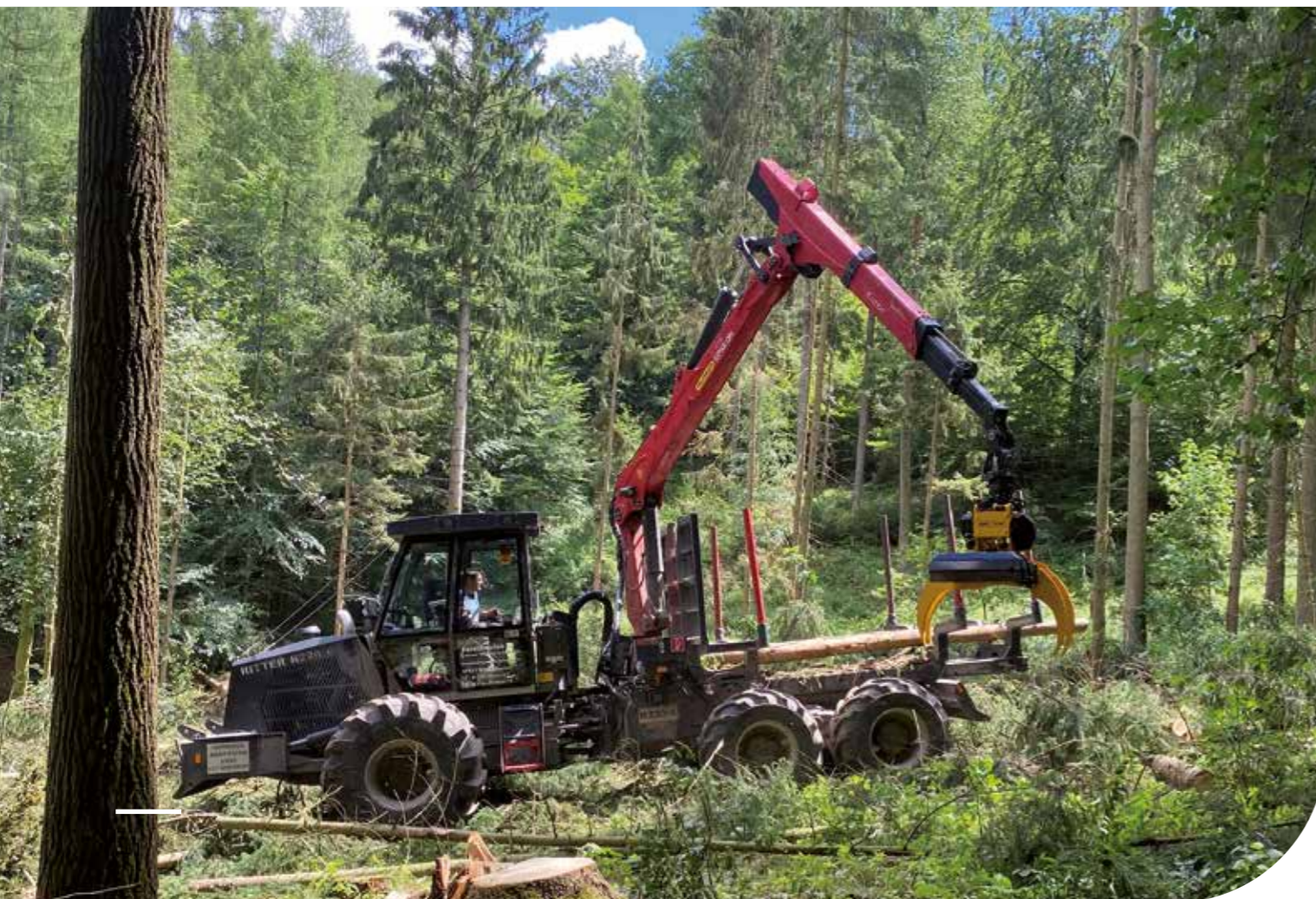
Ritter skidder with a GMT050 grapple saw and GMT C10 quick coupler system
