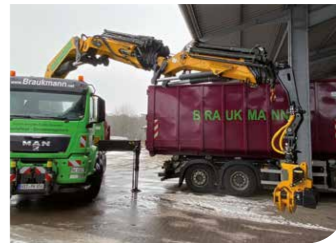
GMT050TTC with extension arm for a knuckle boom crane
